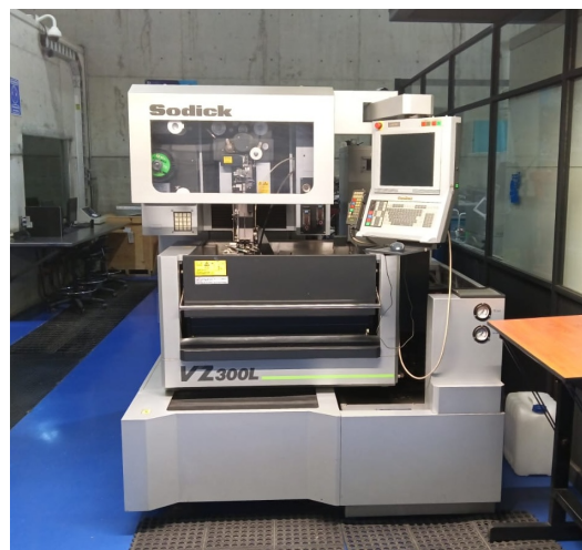
Figure 3. Sodick VZ 300L Wire EDM machine used for the experiments.
