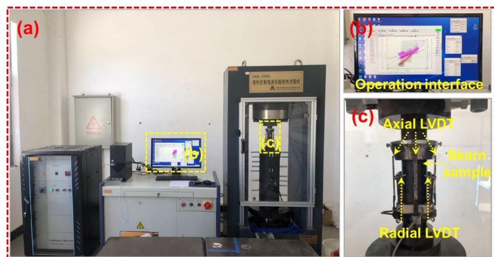
Figure 3. Experimental setup: (a) overview of the test loading system; (b) control interface of the operating system; (c) schematic of the installation of the system for measuring the deformation of rock samples.
