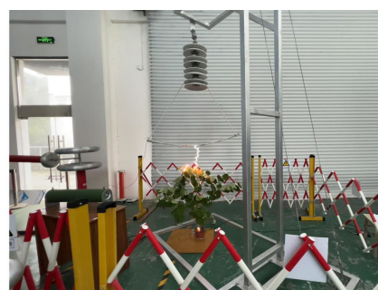
(b) Mid-stage of tree-flash discharge
