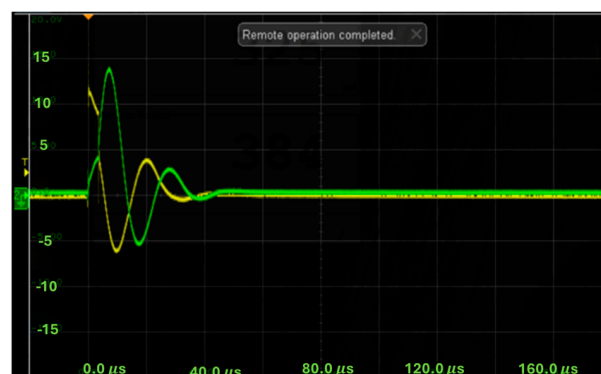
Figure 17. Volt (yellow) and current (green) waveforms of plasma generated in the confined limestone sample.
