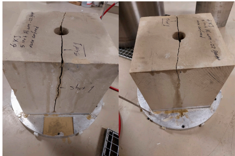
Figure 5. Plasma-propagated fractures after second shot—unconfined sandstone sample.
