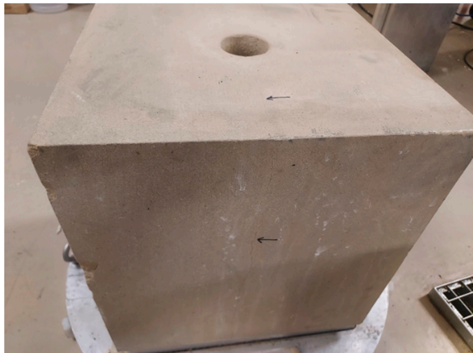
Figure 4. Plasma-propagated fractures using first pressure pulse—unconfined sandstone sample.
