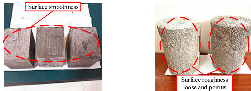
Figure 5. Inorganic cementing material appearance.
