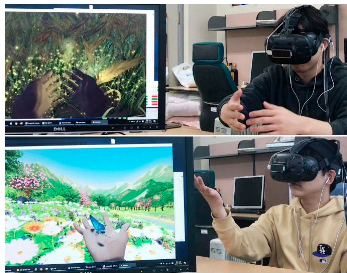
Figure 2. The setup for gesture-based interaction using HTC VIVE and Leap Motion. Users interact with fireflies ( top ) and a butterfly ( bottom ).
