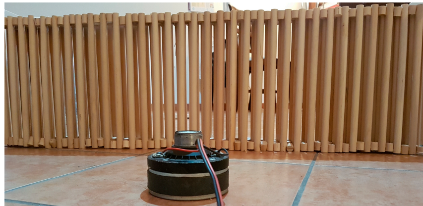
Figure 3. Scale model of metamaterial acoustic barrier.
