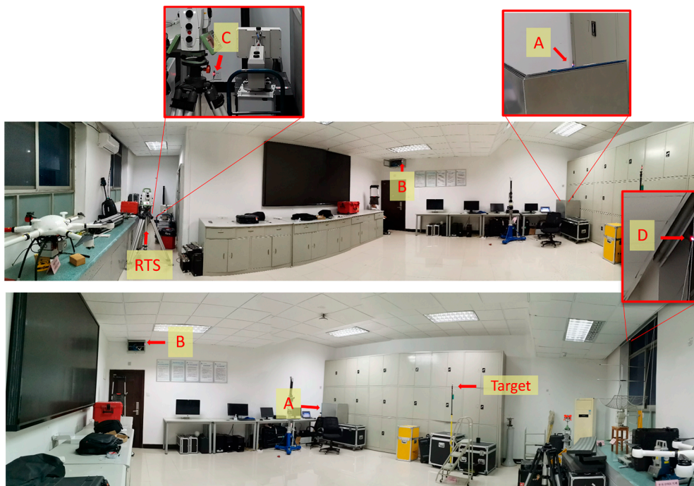
Figure 5. The panorama view of the experimental scene. A, B, C, and D each denote a distinct UWB base station.
