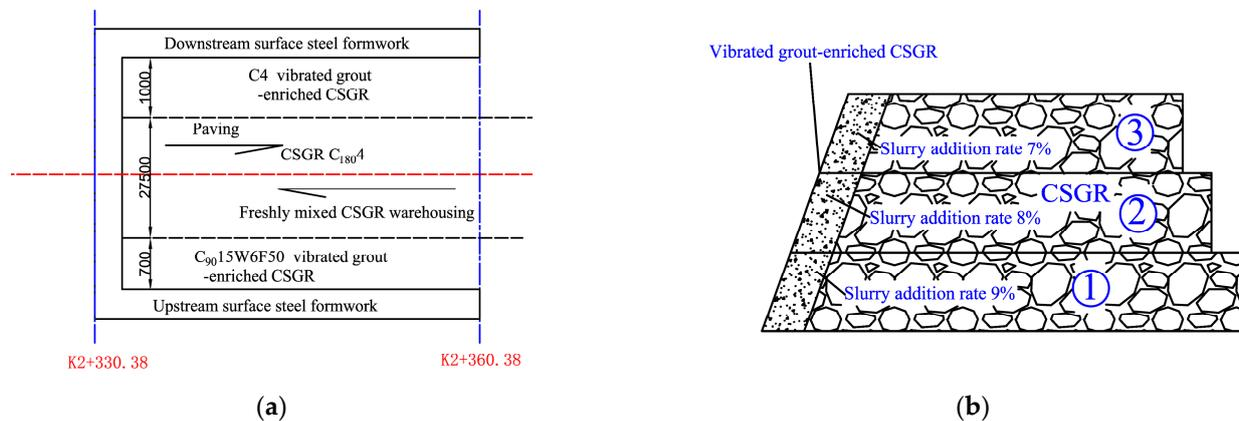
**Figure 11.** The layout of the field test of vibrated grout-enriched CSGR: (a) test area (b) slurry adding test scheme.
