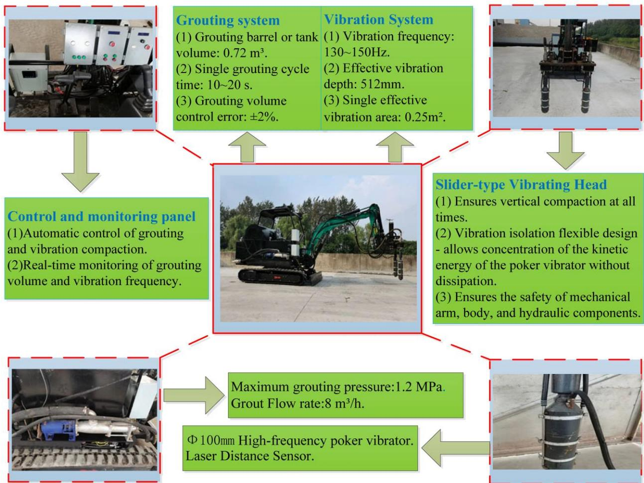
Figure 8. The grouting and vibrating equipment of CSGR.
