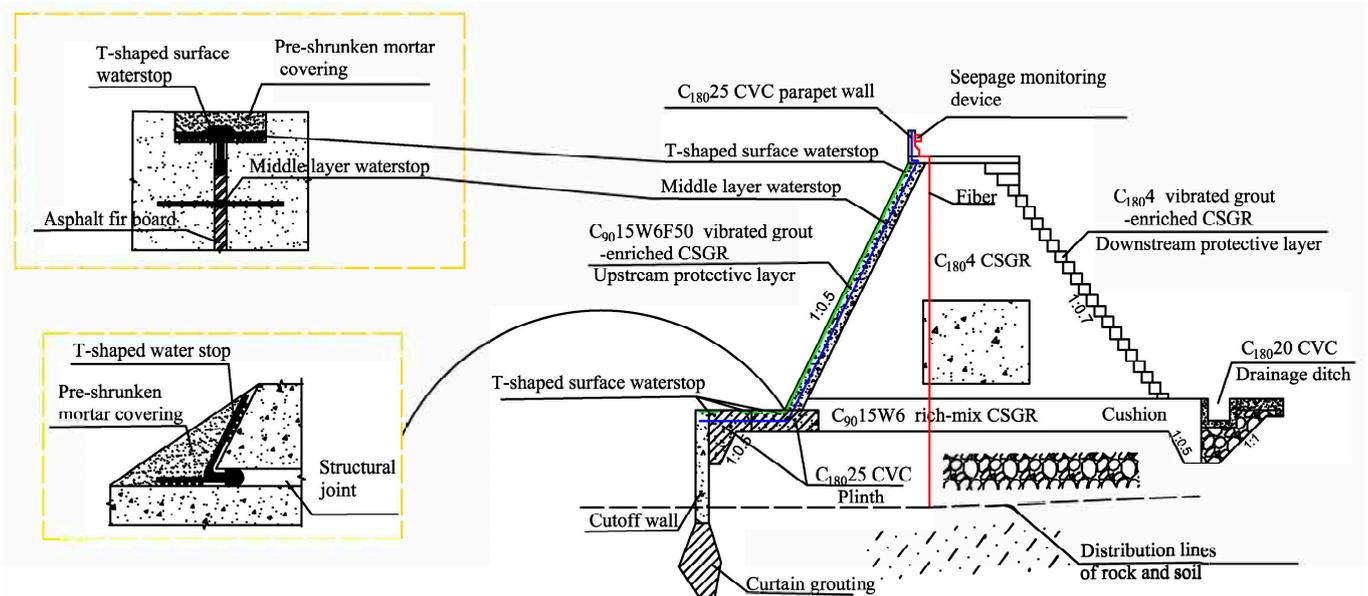
**Figure 3.** The cross-section of Tangba protection dam.
