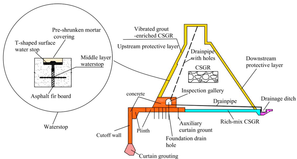
**Figure 1.** New cross-section of CSGR dam.
