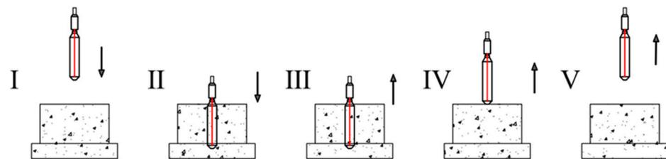
**Figure 9.** Working state of grouting and vibrating equipment (I is the ready stage, II is the insertion stage, III is the grouting and vibrating stage, IV is the redraw stage and V is back to the ready stage for the repetitions of the cycle).
