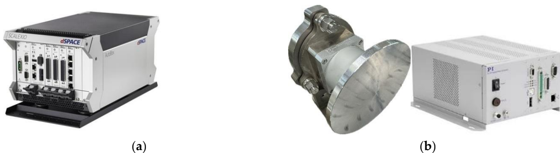
Figure 2. Configuration of fast steering mirror (FSM) platform: (a) Scalexio AutoBox (dSPACE) and (b) tip-tilt actuating platform (PI Ceramic GmbH).
