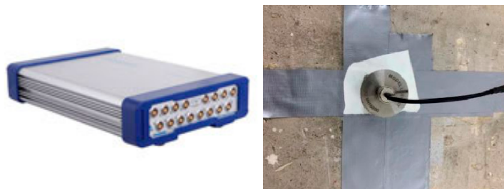
Figure 11. Data acquisition instrument and acceleration transducer.
