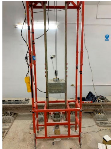
Figure 10. Automatic drop hammer equipment.
