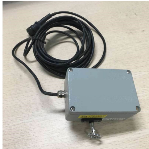
Figure 8. Guyed displacement sensor.
