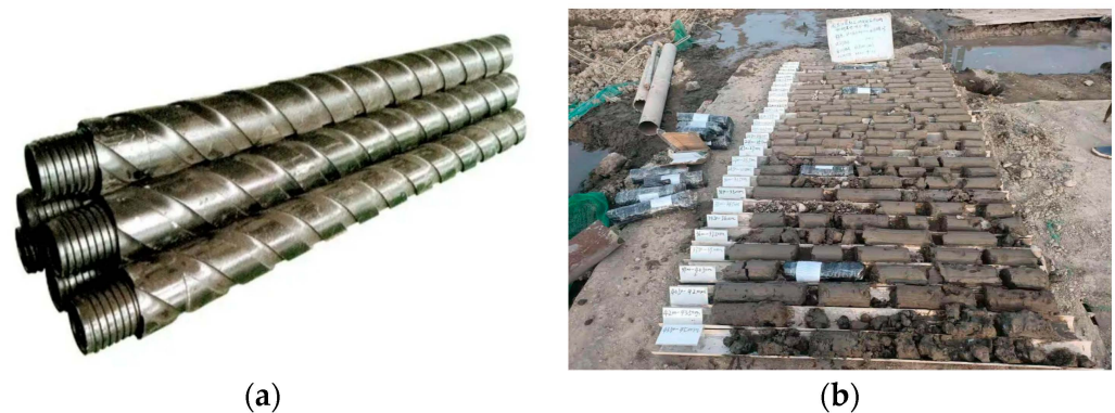
Figure 8. Core samples obtained by drilling for lab tests: (a) Drill pipe for coring. (b) Core samples of waterproof curtain.
