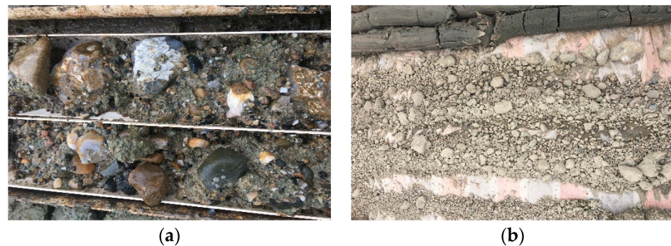
Figure 2. Representative core samples of ⑤-1 and ⑤-2 layers: (a) Core samples of pebble gravel. (b) Core samples of gravelly sand.
