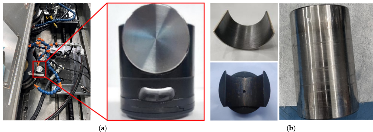
Figure 1. Test rig installation diagram: (a) test specimen and friction pair test bench; (b) 15% SCF/PEEK modified bearing bush and friction pair accessory.
