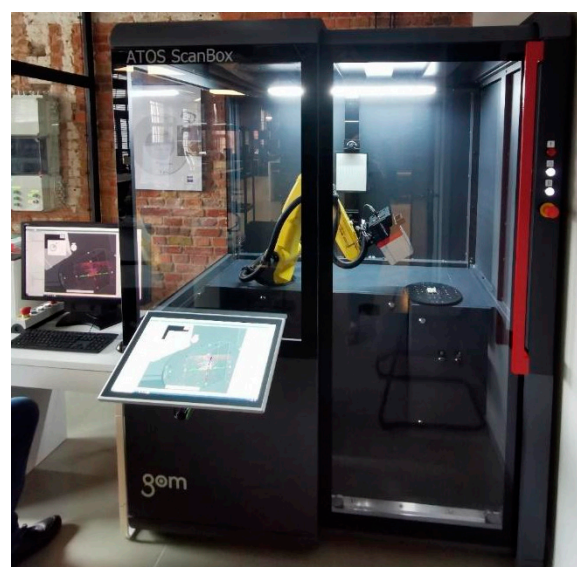
Figure 3. ATOS ScanBox Series 4 measurement station.
