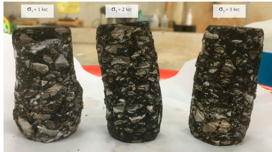
Figure 7. Test sample condition of Mix Proportion 1 after triaxial compression test.
