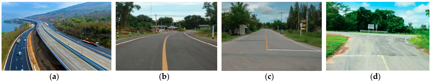
Figure 10. Examples of road profiles for classes A to D: (a) class A, (b) class B, (c) class C, and (d) class D.
