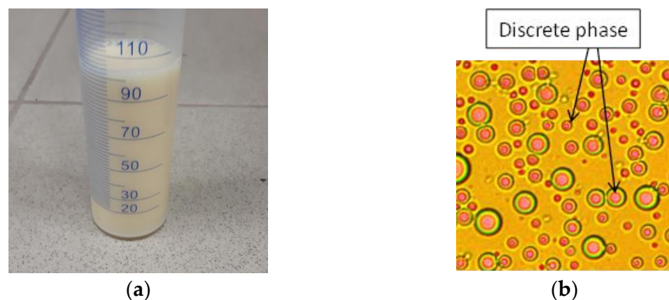
Figure 8. Photo of the fuel–water emulsion: (a) macroscopic; (b) microscopic.
