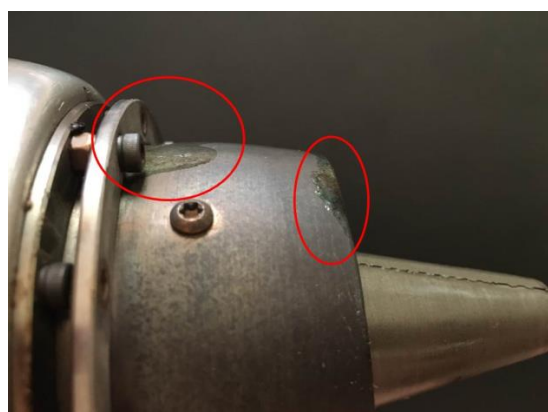
Figure 18. GTM120 gas turbine outlet nozzle with the marked places indicating glassy deposits.
