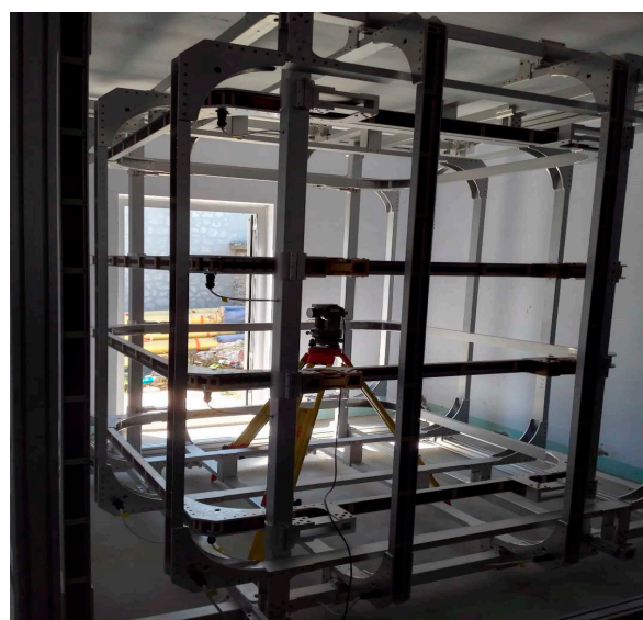
Figure 23. Ultra-high-uniformity magnetic field generation system.
