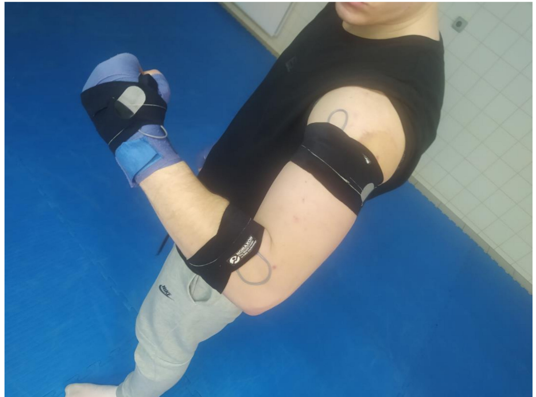
Figure 1. Placement of IMU sensors on upper limb.
