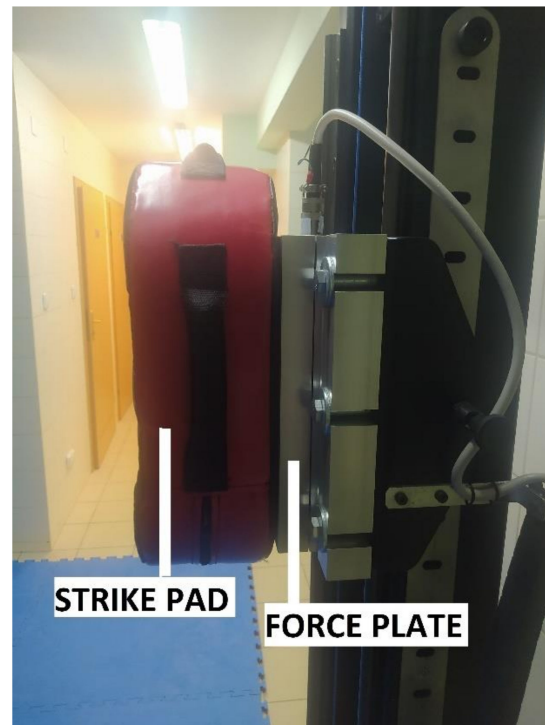
Figure 2. Force plate AMTI MC12-2K with a strike pad.
