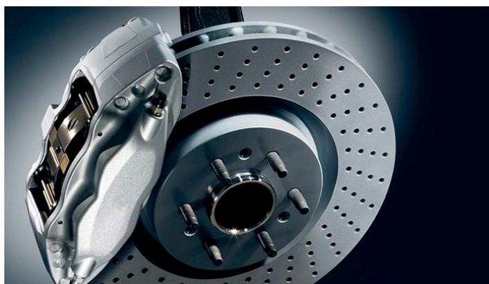
**Figure 1.** Disc brake with a fixed caliper [40].
