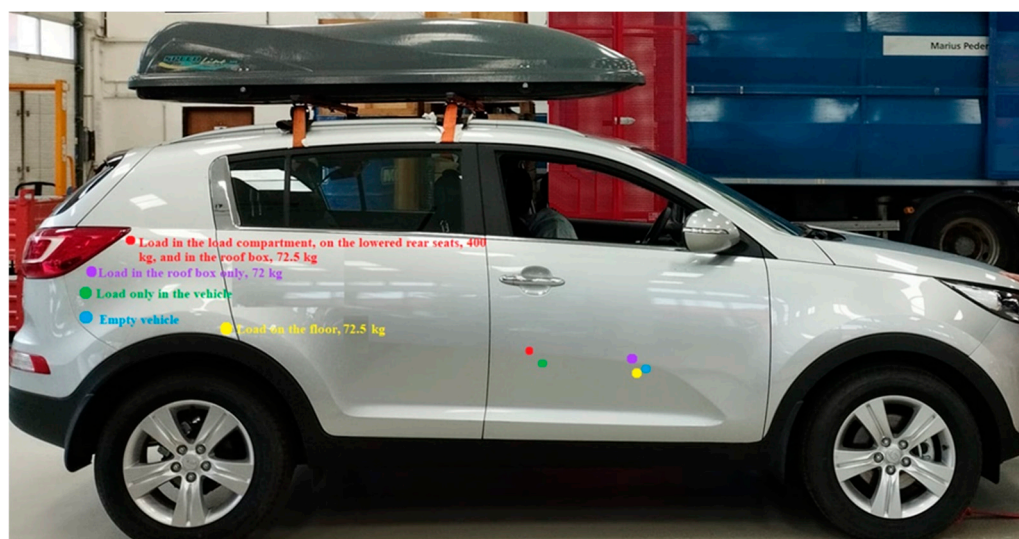
Figure 8. Position of the center of gravity of SUV.
