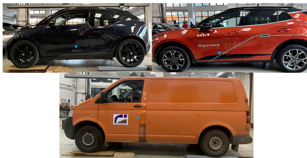
Figure 9. Position of the center of gravity of electric, hybrid, and VAN.
