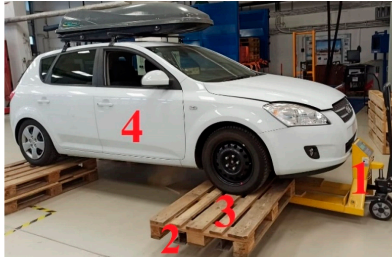
Figure 2. Principle of determining the axle load via the weight scale pallet truck in the horizontal direction.
