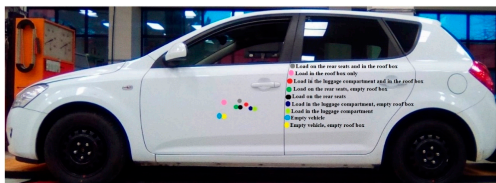
Figure 7. Position of the center of gravity of hatchback.
