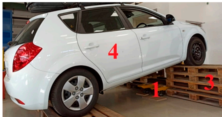
Figure 3. Principle of determining the axle load via the weight scale pallet truck in the vertical direction.
