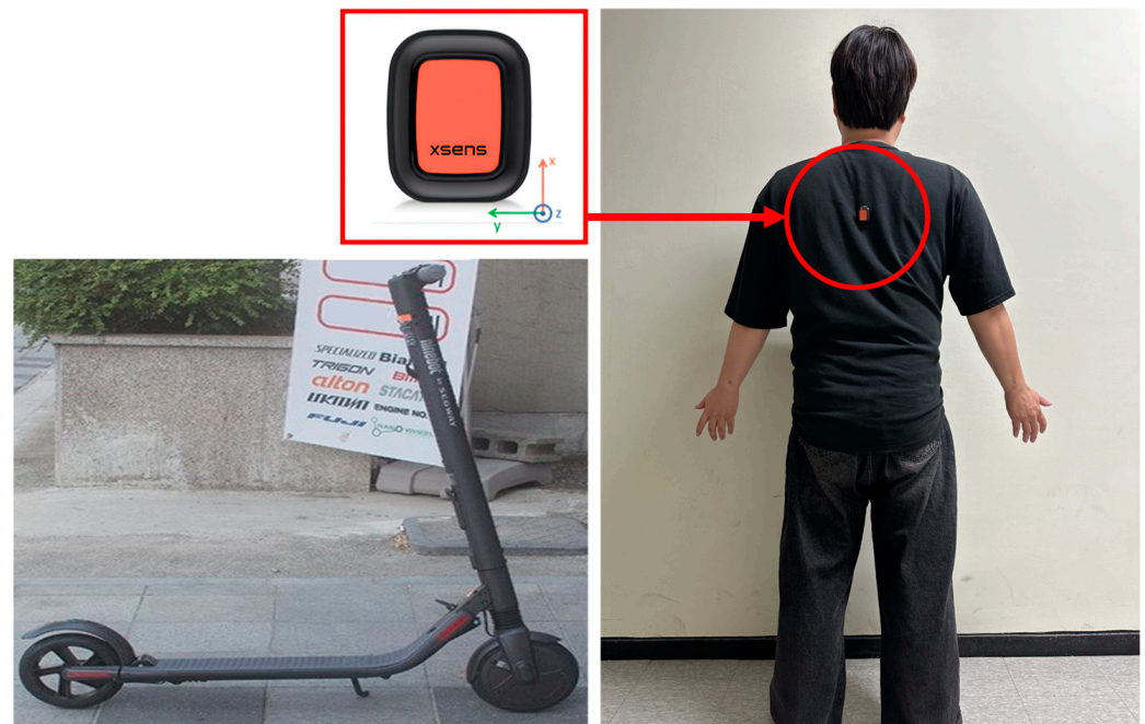
Figure 1. The e-scooter and an IMU sensor (position: T7).
