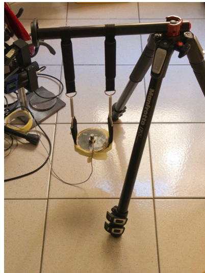
Figure 6. Calibration structure for setup calibration using elastic supports.
