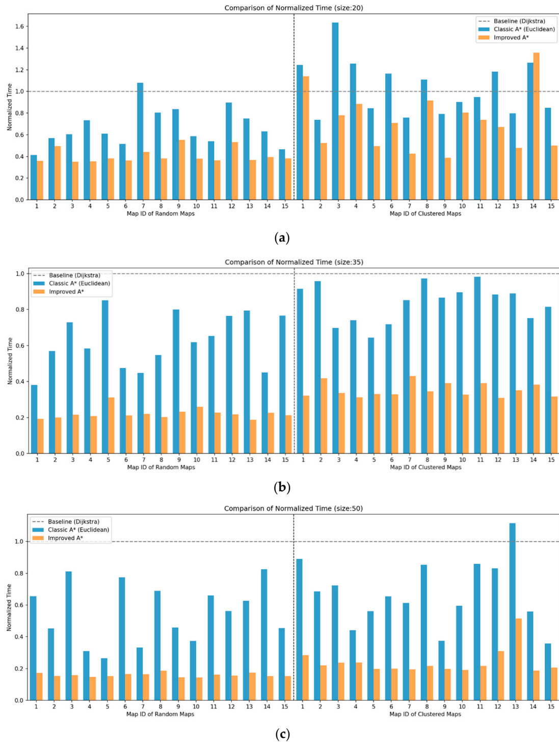
Figure 6. Comparison of running time between the SSA-A* and Classical A* Algorithms. (a) corresponds to the 20 \times 20 grid map, (b) corresponds to the 35 \times 35 grid map, and (c) corresponds to the 50 \times 50 grid map.
