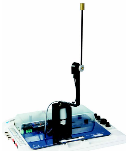
Figure 11. Inverse rotary pendulum system.
