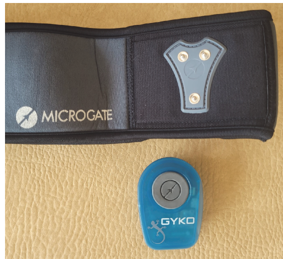
Figure 1. IMU sensor device (Gyko, Microgate, Bolzano, Italy).
