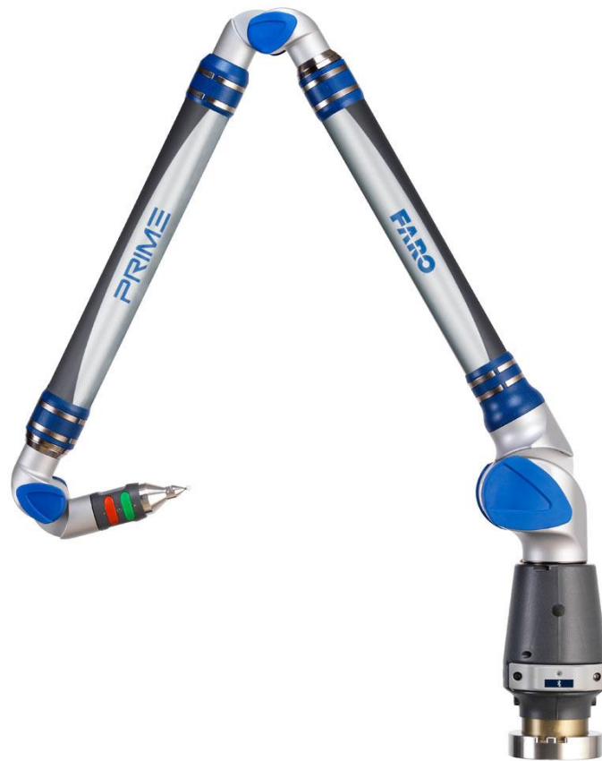
Figure 11. FARO Prime 3D Arm.
