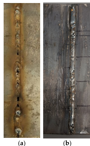
Figure 7. Visual inspection of the WAAM specimen: (a) after root pass, showing early pore formation, and (b) after three passes, with visible porosity clusters confirming successful defect seeding.
