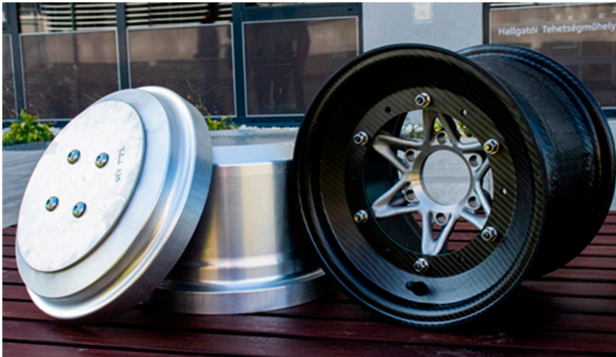
Figure 1. ART's previously used a three-piece CFRP rim and its laminating tools.
