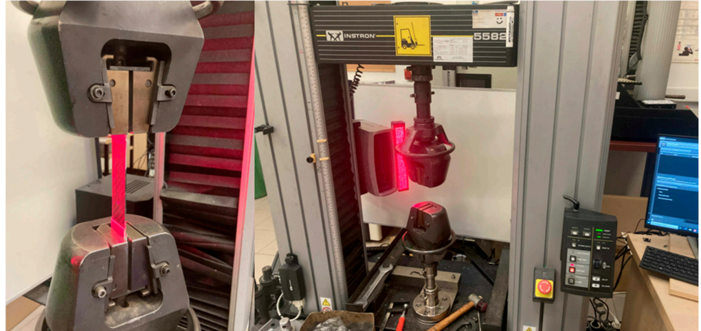
Figure 6. Tensile testing machine with the specimen. The tests were conducted at 2 mm/min and at a constant 20 °C room temperature.
