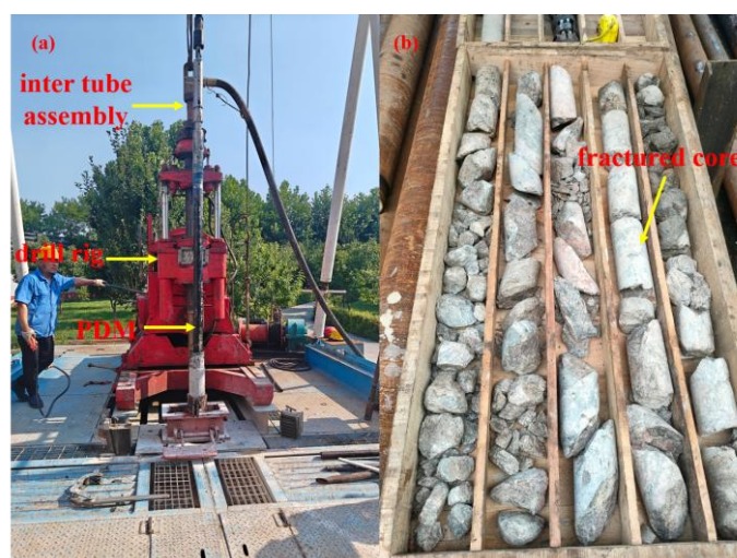
Figure 16. Core drilling tests and recovered core samples.
