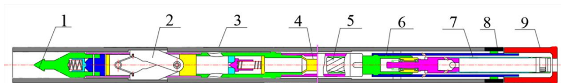
Figure 1. The structural diagram of a DCDT. 1—fishing tool; 2—latch head assembly; 3—nonmagnetic outer tube; 4—measurement while drilling system (MWD); 5—small-diameter and high-torque PDM; 6—torque transmission tube; 7—high-strength core barrel; 8—HSBS; 9—core bit.
