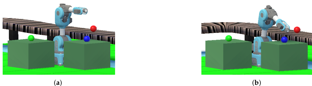
Figure 12. Representative manipulator postures (a) before and (b) after GA-based posture optimization. The optimized configuration reduces collision risk and minimizes the total motion required to reach pick, place1, and place2 targets.
