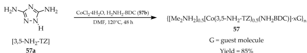
Scheme 45. Synthesis of a cobalt-based framework ( 57 ) using 3,5-diamino-1,2,4-triazole ( 57a ) and 2-amino-1,4-benzenedicarboxylic acid ( 57b ).
