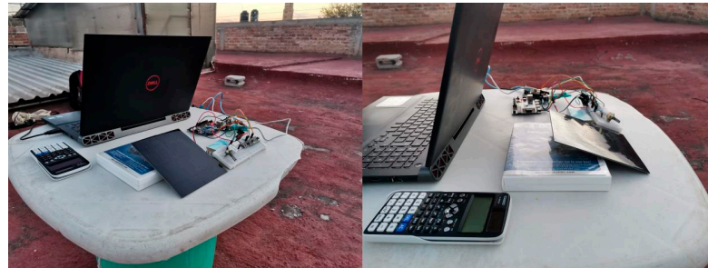
Figure 13. FPGA-based solar radiation sensing and measurement system.
