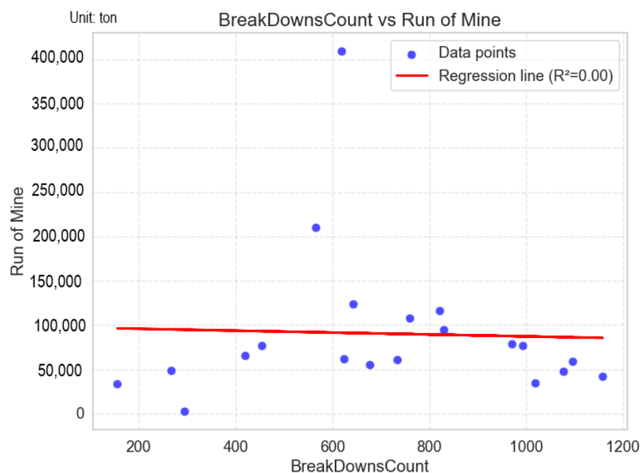
Figure 6. Relationship between breakdown counts and Run-of-Mine quantities ( R^2 = 0.001 ), illustrating negligible linear association.
