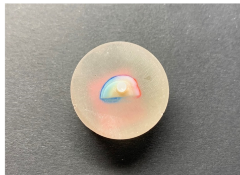
Figure 1. Sample prepared for shear bond testing. Dentin slab embedded in acrylic resin with composite cylinder.
