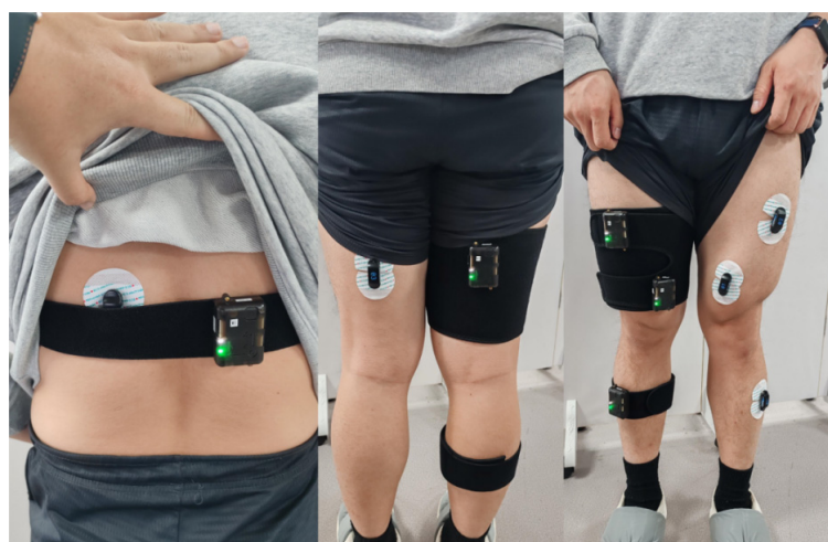
Figure 6. Schematic diagram of sEMG and MMG sensors in human measurement position.
