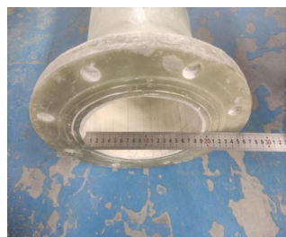
Figure 4. Finished alumina wear-resistant chute pipe.
