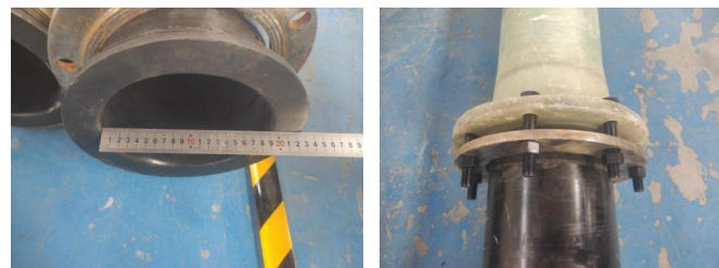
Figure 8. Ultra-high polymer wear-resistant chute joint adopts flange connection.
