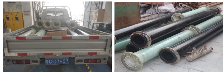
Figure 17. The finished product of the wear-resistant tube.
