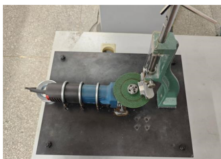
Figure 10. Schematic diagram of the grinding wheel wear test apparatus.
