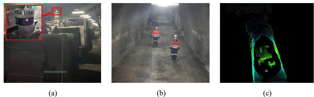
Figure 11. Specifics of the underground mine personnel dataset: (a) the Ouster OS1 mounted on top of a shovel loader, (b) a 2D image frame of the underground mine dataset captured by cameras, and (c) a 3D point cloud image frame of the underground mine dataset captured by LiDAR.
