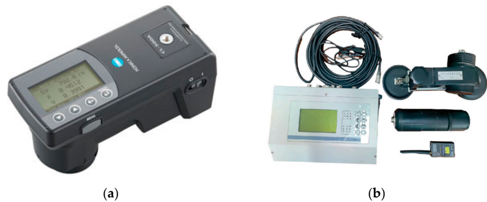
Figure 10. Test instruments and equipment. (a) Spectroradiometer, (b) Non-contact multifunctional speedometer.
