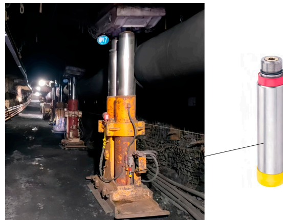
Figure 1. Installation position of the safety valve on the hydraulic support.
