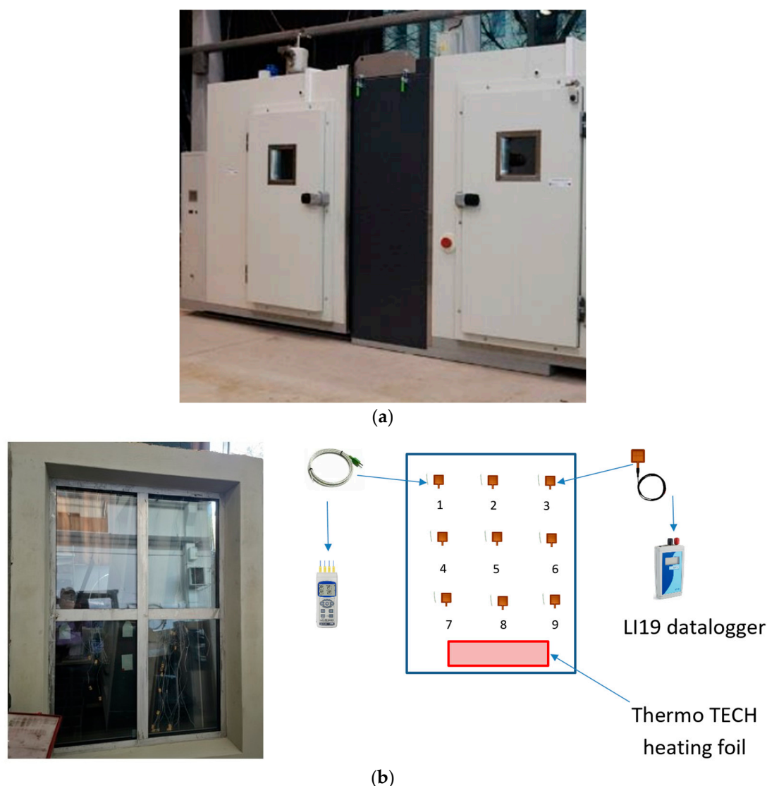
Figure 9. Experimental setup for active glazing thermal performance evaluation: (a) the dual-zone climatic chamber; (b) active glazing heating system, including thermometer TM-947SD, hukseflux
