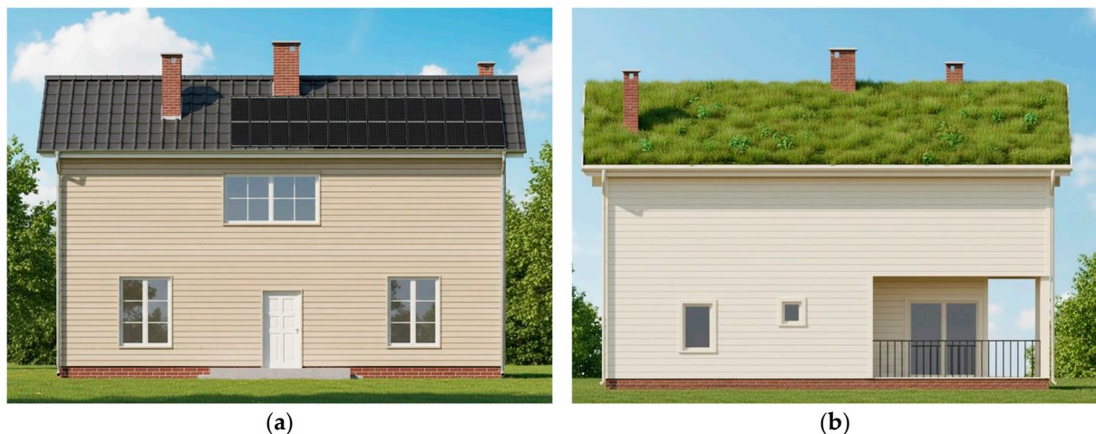
Figure 15. Architectural transformation and technical integration of the building envelope following the NZEB adaptation: (a) Eastern elevation showcasing the integrated 7 \text{ kWp} polycrystalline photovoltaic array and modernized pine wood cladding; (b) Western elevation demonstrating the nature based cooling strategy via the extensive green roof system and the elimination of thermal bridges through the removal of legacy balcony structures.
