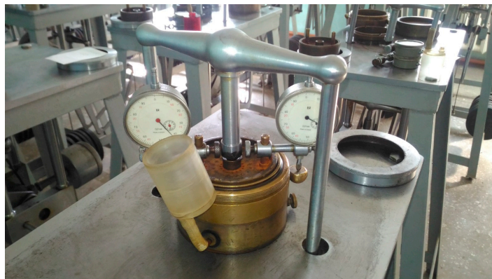
Figure 5. Soil Sample under Compression in the KPr-1M Apparatus.
