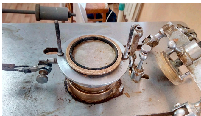
Figure 6. Tested soil specimen under shear.
