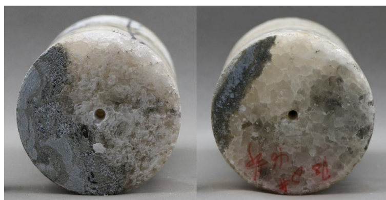
Figure 1. Surface morphology at the drilled specimen end.
