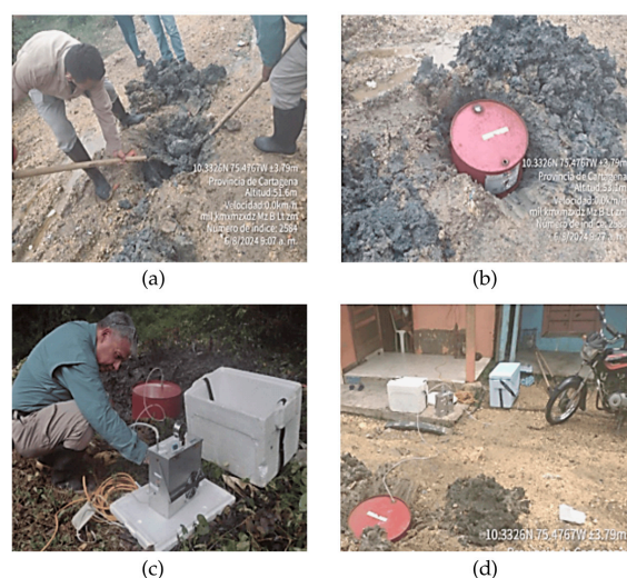
Figure 5. Field procedure for gas sampling. (a) Equipment setup for installation of the extraction system; (b) Placement of the inverted chamber for gas collection; (c) Calibration of the vacuum pump; (d) Automated gas extraction process.
