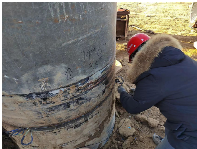
Figure 4. Connecting sensor signal cables.
