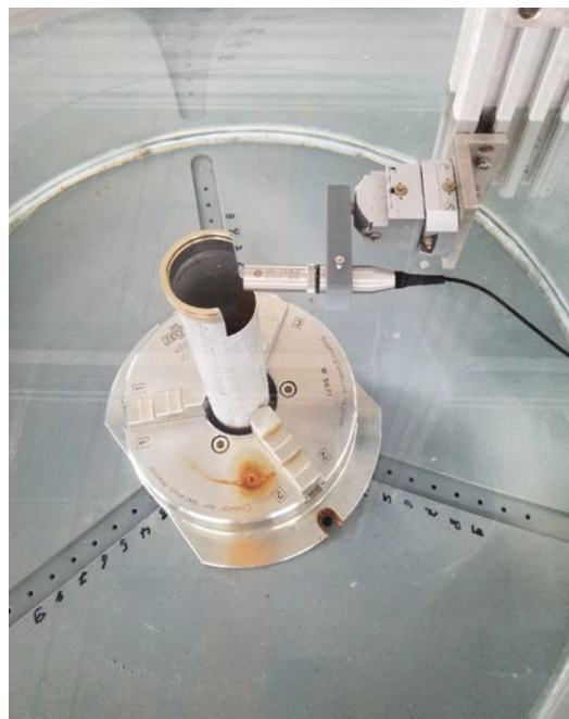
Figure 8. Measurement setup for runtime measurements with a single sensor from the inside of the pipe.
