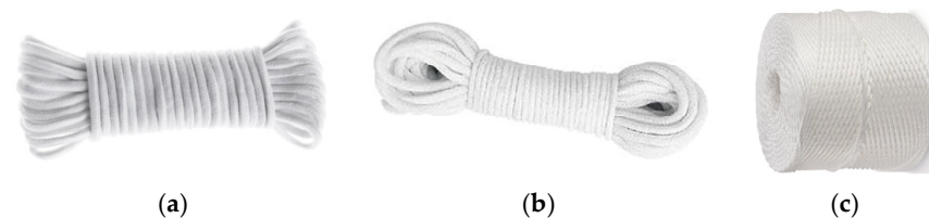
Figure 6. Specifications of the tested cords: (a) polyester fibre with a width of 10 mm; (b) polyester fibre with a width of 6 mm; (c) polypropylene cord with a width of 2 mm.
