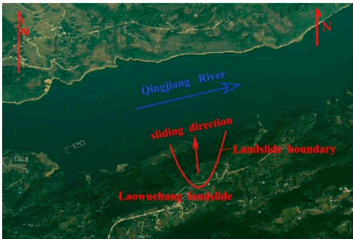
Figure 2. Plan View of the Laowuchang Landslide.
