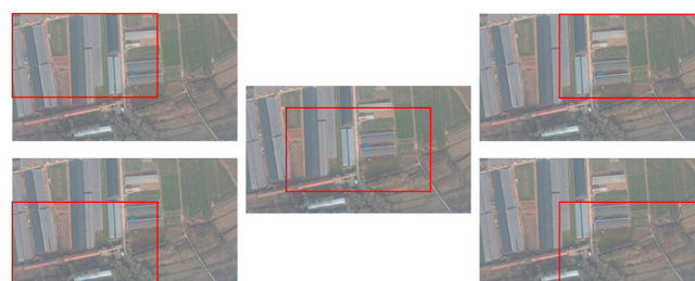
Figure 1. The multi-region annotation of five keypoints. The red boxes indicate different regions where keypoints are selected.
